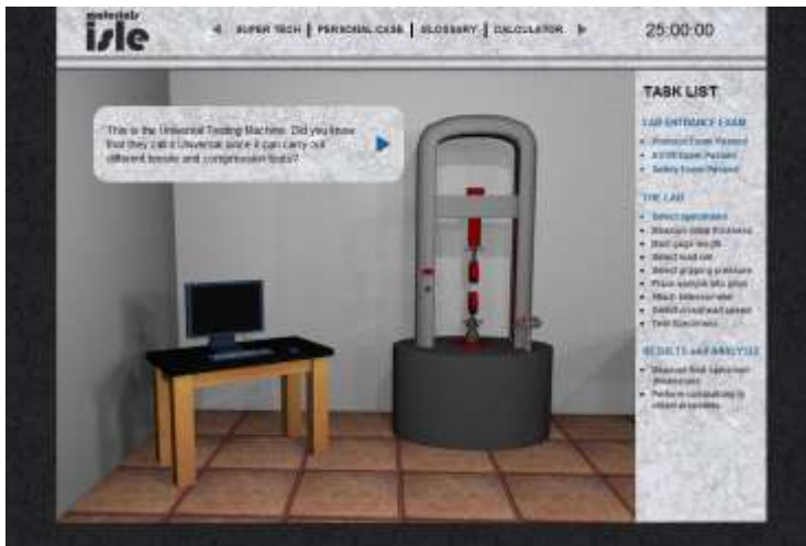
Fig 3: The Virtual Tensile Testing Machine
