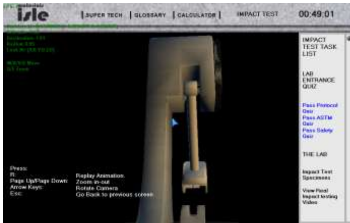
Fig 8: Simulated swing of Impact Test Machine through the sample
