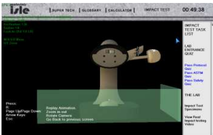
Fig 7: Safety glass comes up to simulate sheltering user from flying fragment
